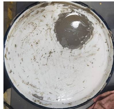
Final printed shape after draining flowable GGBS 4M
